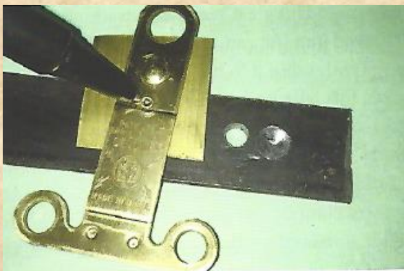
Rivet is now ready to be set against the bridge by peening. Note that the tungsten point is hanging just off of the side of the buck
