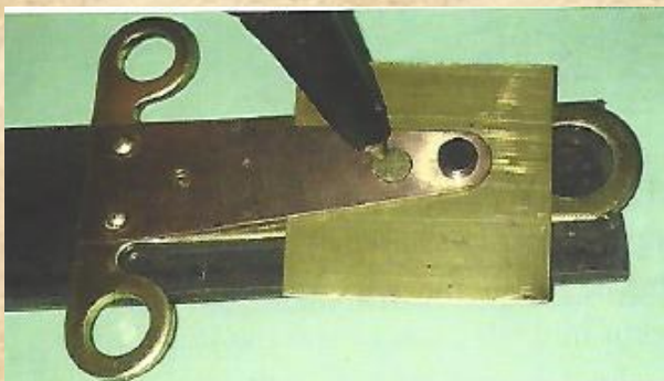
Bridge on the rivet buck. Brass rivet is ready to be gently tapped with a punch until the shim is snug.
